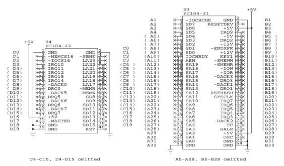
The DB implements a subset of the PC/104 specification in the form of two connectors that provide only +5V and GND for PC/104 modules. Only a total of 32 pins are implemented, 16 on H3 and 16 on H4. By adding up to four 8-pin connectors to the DB, PC/104 modules can be plugged directly into the DB to obtain +5V power and GND. No other connections between the PC/104 bus and the CubeSat Kit Bus are provided.
